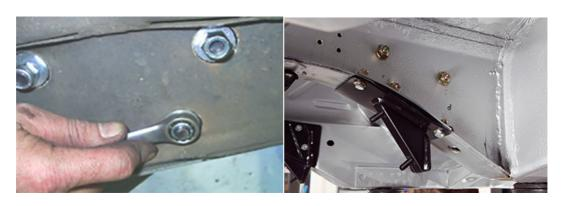
The Steering box nuts and bolts torque settings are 40ftlbs 55nm.
