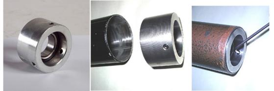
Lower column bearing mount. Lower column bearing mount, being fitted to shortened column. Tighten grub screws to secure in place.
