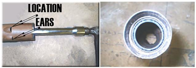
Fit mount into place so that it is 2mm to 3 mm (1/8" to 3/16") past the location ears on the outside of the column. The mount in place should look like this. Then reassemble the entire column ready for the installation of the RRS lower column shaft and bearing mount.
