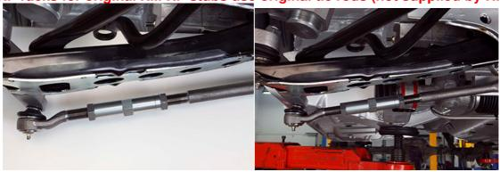
STEP 13: Tie rod end adjusters must be adjusted to allow equal range of movement (rack is centred). The linear tacking is pre-adjusted and is offset. *Do not use the linear tracking as guide to centre.* With the outer tie rods not connected turn the wheel to full lock then full lock the other way, calculate centre (half the lock to lock turns).
