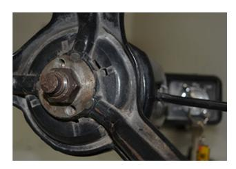
Internally is another telescopic tube through which the steering shaft passes. The upper internal shaft and upper bearing remain unchanged.
