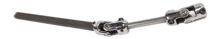
RRS lower column shaft, upper uni., intermediate shaft and lower uni.
