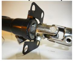
The column is now ready to fit back into the vehicle.
