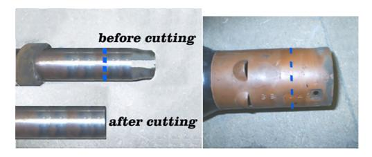
It is necessary to completely dismantle this type of column so that the inner tube can be shortened approx. 3.5". The end of the outer column that protrudes through the firewall must be shortened approx. 1 ½ inches or flush to the fire wall.
