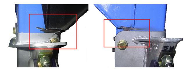
STEP 6: Install RRS conversion brackets onto the chassis rails and torque bolts to specified settings.
