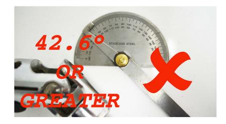
Correct uni-joint alignment is achieved when both uni-joints are at the same angle, and that angle is 42.5° or less.
