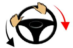
Once level has stabilized, check turning is smooth and system is running quietly, you are ready to take the car for wheel alignment.
