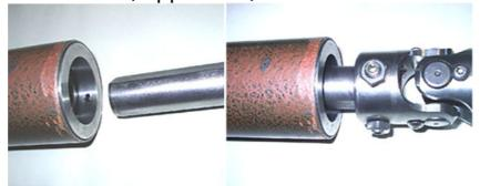
Slide RRS lower column internal shaft into bearing housing engaging at least 5" of upper shaft. Column end should look like this after installation. Refit steering column, anchor lower column mount in such a way that no universal bind occurs.
