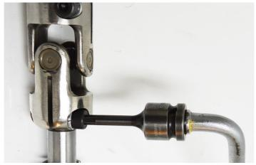
Step 17: The universal joint alignment is determined by adjusting the steering column position in the firewall opening.
