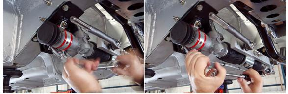
STEP 12: Connect tie rod ends making sure adequate thread engagement into sleeve.
