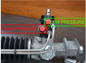
If you are fitting a powered rack it is easier to fit the hydraulic lines before bolting the rack in place.
