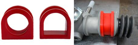
STEP 10: Fit U clamps around rack rubber and fit to up to rack checking alignment is correct to rack. If rack does not line up stop and call RRS.
