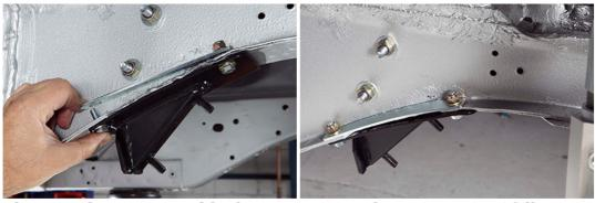
The load spreader nuts and bolts torque settings are 18-20ftlbs 22-24nm.
