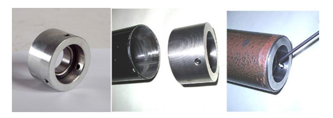
Lower column bearing mount Lower column bearing mount, being fitted to shortened column. Tighten grub screws to secure in place.
