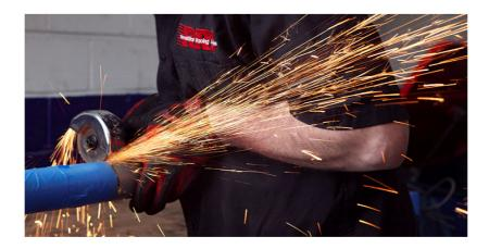
Cut column to length, de-burr and clean cut, remove scam ridge if necessary.
