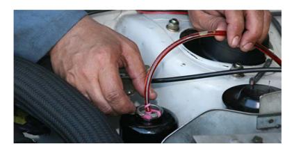
Once you can can turn the wheel lock to lock and the level is unchanged, start the vehicle momentarily. Turn off the vehicle and check level again. Add power steering fluid if the level is low.
