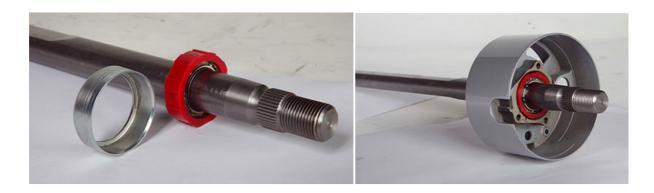
RRS upper internal column shaft and locater bearing and collar.RRS upper internal column shaft and locater bearing and collar fitted to top of the column. **NOTE**: on some vehicles steering wheel to blinker housing interference may occur, this can be remedied by either cutting back the die cast blinker shroud or cutting new cir-clip grooves in the steering shaft further down.
