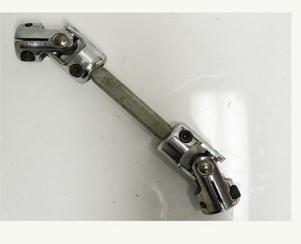
If the column is too low or too high in the firewall uni-joint misalignment will occur causing uni-joint bind with typical feel of notchiness or a binding spot as the steering wheel is turned.
