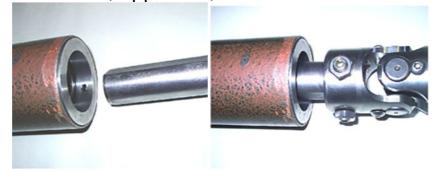
Slide RRS lower column internal shaft into bearing housing. Slide RRS lower column internal shaft into bearing housing engaging at least 75ml of upper shaft.
