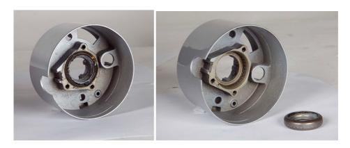
Once column is removed, cleaned and dismantled remove top bearing and casing. The inner bearing case must be separated from the outer bearing case, which may require grinding the inner case to enable it to be separated easily.
