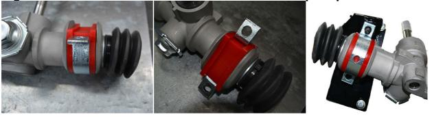
STEP 11: Install rack tighten until rack is firm against mounting bracket
