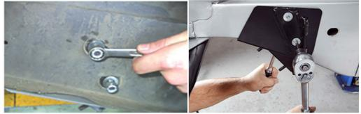
The Idler nuts and bolts torque settings are 30ftlbs 38nm.
